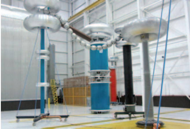
Fig. 3 Insulating case transformer cascade type WP 1000/1000
