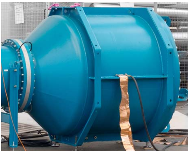
Figure 1: Test transformer, type PEG 500/750
