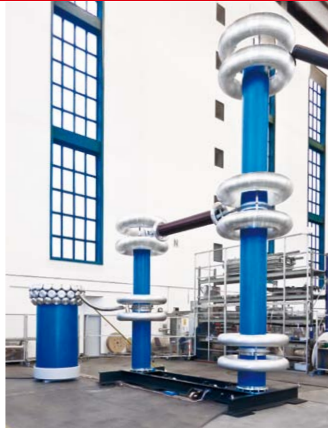
Fig. 2 HVDC power supply type GE 200/900
