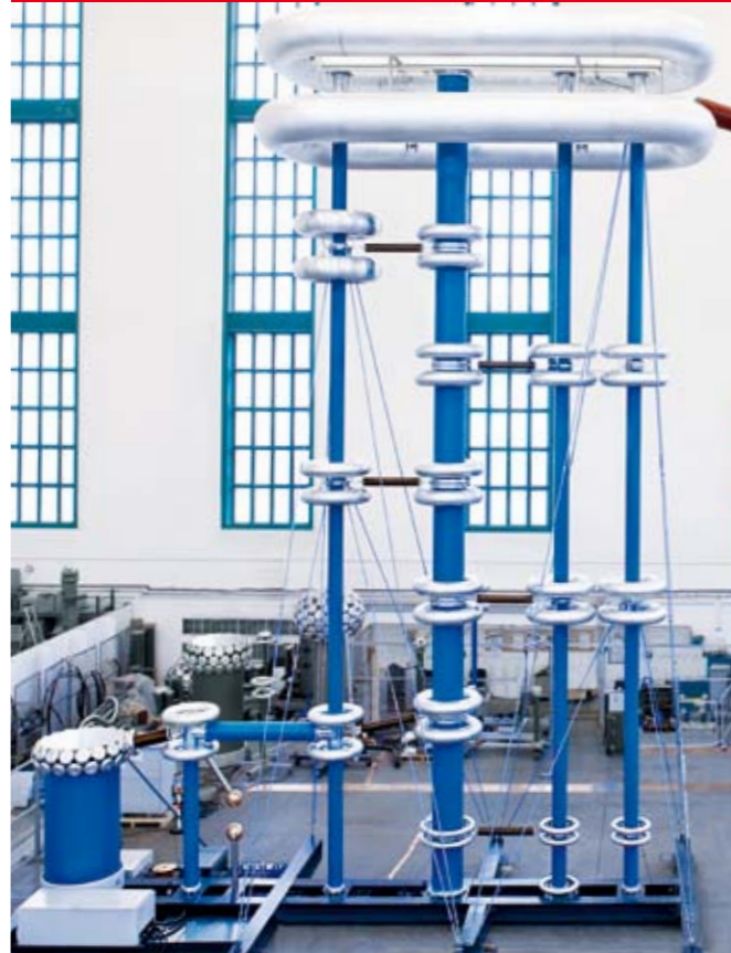
Fig. 1 HVDC test system type GP 50/2000
