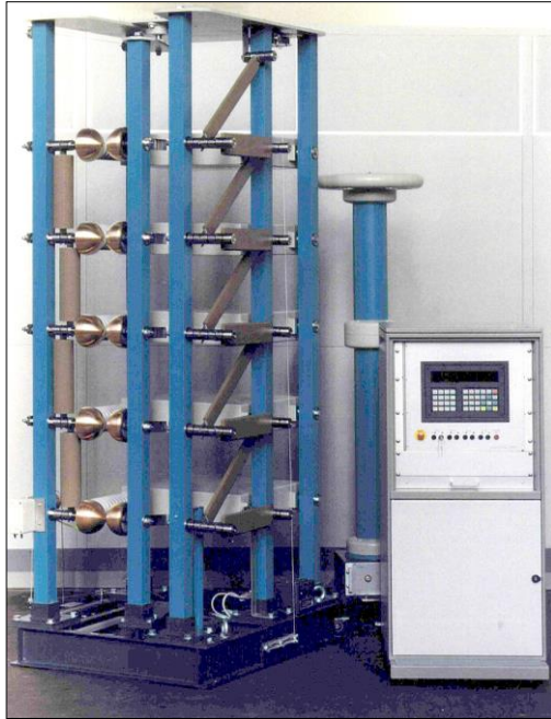
Figure 1: Impulse voltage test generator IG 10/500 L
