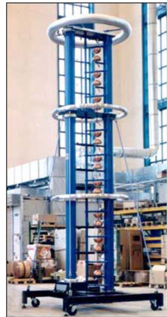
Figure 2: Chopping gap of a maximum chopping voltage of 1800 kV
