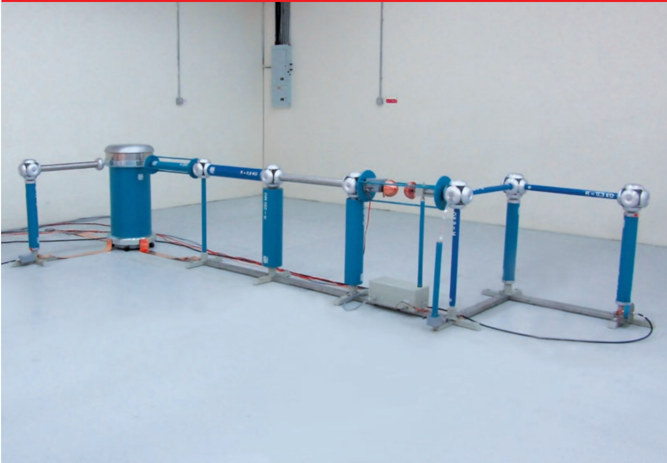
Fig. 1 Combined AC, DC, and impulse test system, type WGSBS 5.8/100-135-135, 100 kV AC, 135 kV DC, 135 kV impulse voltage
