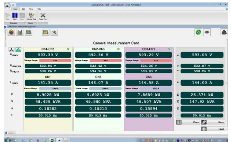
Figure 2: Transformer Loss Measuring System LiMOS MS 1000/5-3 (left: rack arrangement; right: software iMOS)
