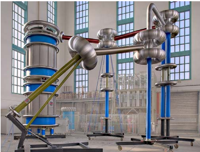
Fig. 1: Shielding and connection electrodes of a HV test system
