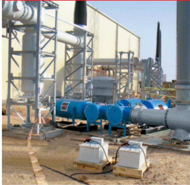
Fig. 1 AC resonant test system type WRVG G for on-site testing of GIS/GIL
