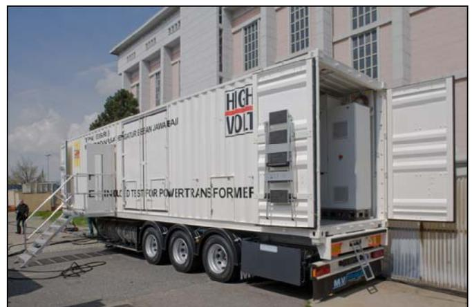
Fig. 4: 40 ft container for transformer test systems
