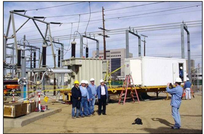
Fig. 3: Combined container on a trailer for HV cable testing (The exciter transformer is arranged inside that container).
