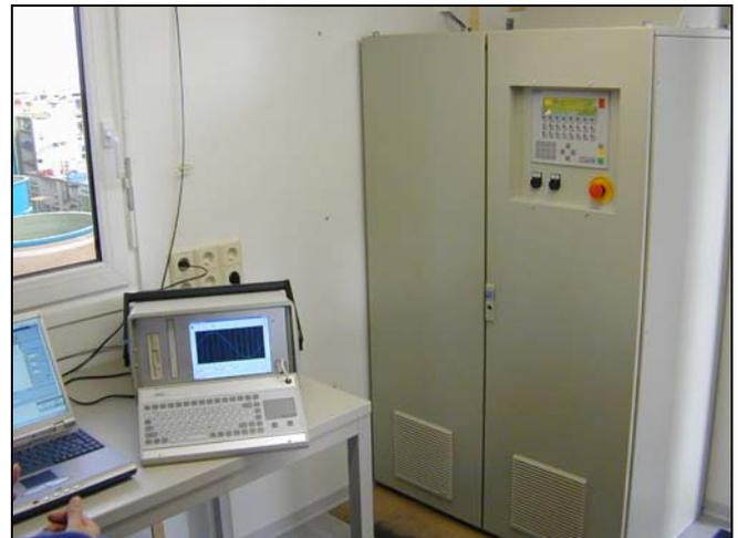
Fig. 1: Inside a control container for a frequency-tuned resonant test system for cable testing
