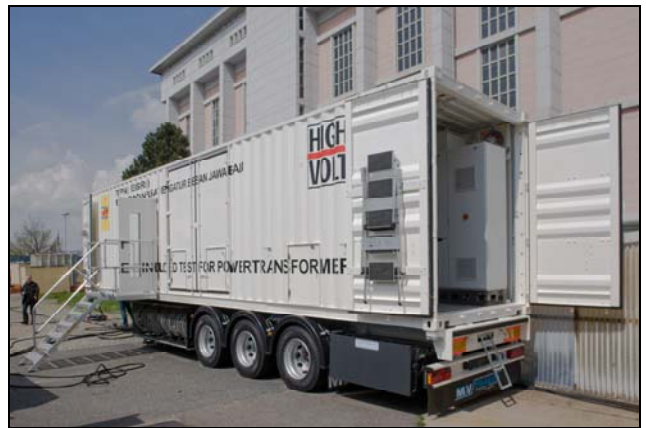
Fig. 6: Container chassis with 40 ft container for transformer test system
