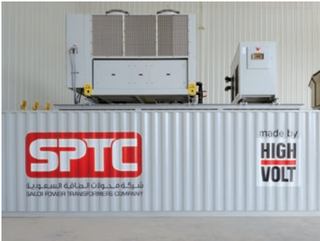
Fig. 3 Test system for medium power transformers (left: test voltage source 1 MW/2 MVA [SFC] in 40 ft container, right: test system 620kW/1MVA + HVCC)
