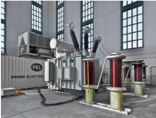
Fig. 4 Test system for large power transformers (left: 2 MW 4 MVA [SFC], step-up transformer and filters, right: loss measuring system LiMOS 2000/100-3)
