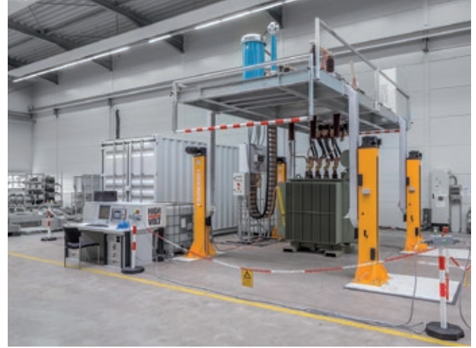
Fig. 1 Test system for routine tests on distribution transformers (left: test voltage source type MWV, right: disconnector lifting platform)
