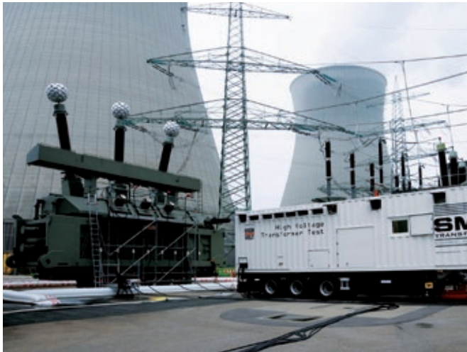
Fig. 4 Test system for on-site tests on transformers (left: WV 620-1000/80, right: extension for applied voltage tests WRV 5/360 M)
