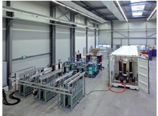
Fig. 3 Test system for medium power transformers (left: test voltage source 1 MW/2 MVA [SFC] in 40 ft container, right: test system 620kW/1MVA + HVCC)
