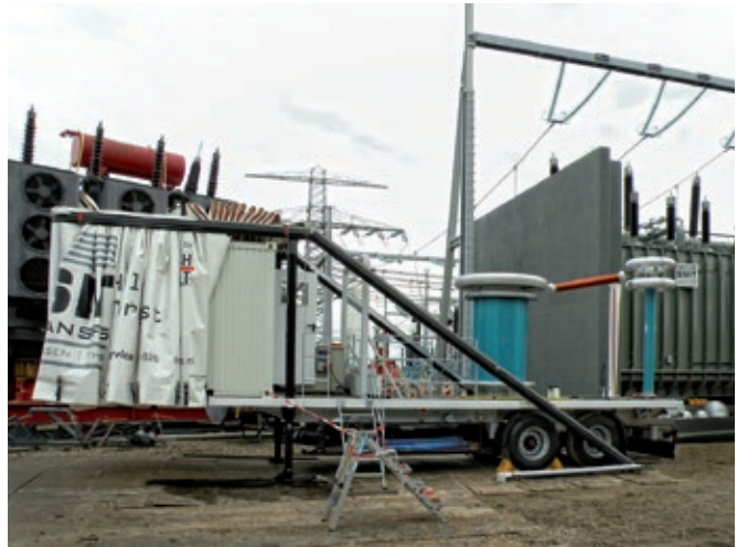
Fig. 4 Test system for on-site tests on transformers (left: WV 620-1000/80, right: extension for applied voltage tests WRV 5/360 M)
