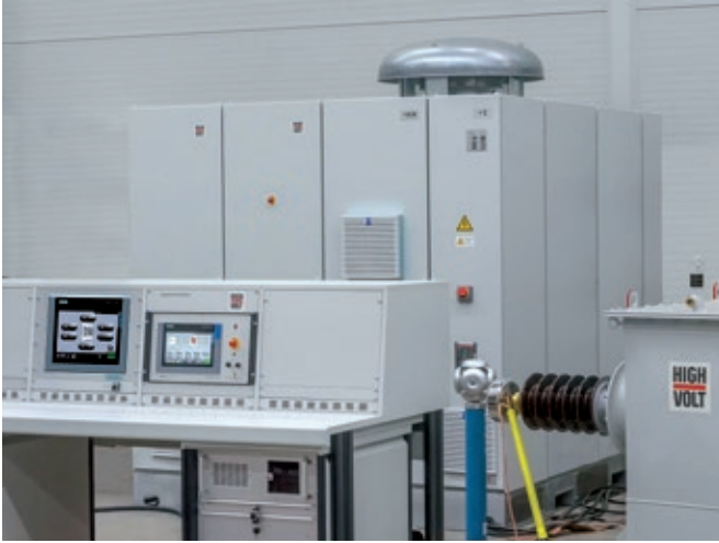
Fig. 1 Test system for routine tests on distribution transformers (left: test voltage source type MWV, right: disconnector lifting platform)
