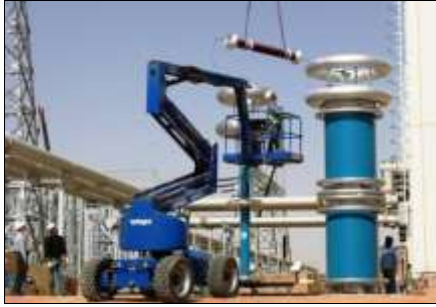
Fig. 3: Modular DC test system type GPM 30/800 (30 mA, 800 kV); continuous operation; Manufactured by HIGHVOLT
