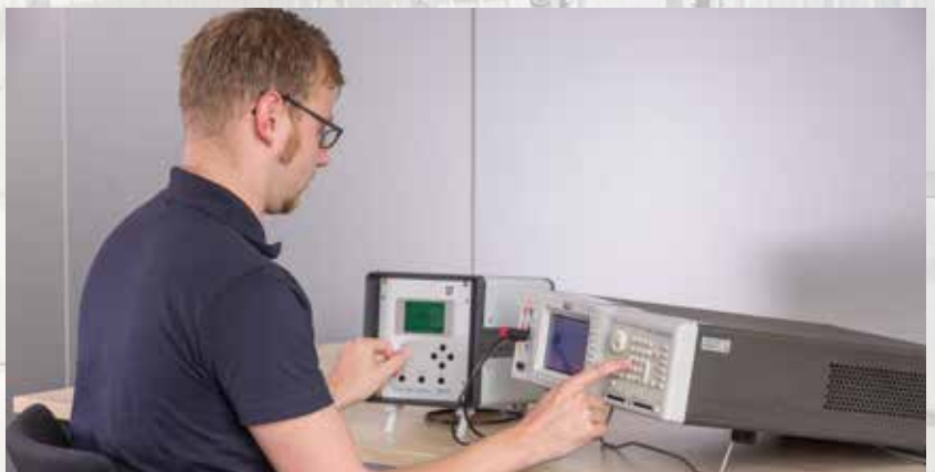
Felix Wolf is calibrating a voltage meter, used for AC and DC voltages, with a calibrator. HIGHVOLT calibration laboratory is certified by Germany's National Accreditation Body DAkkS, according to DIN EN ISO/IEC 17025:2005. The DAkkS is signatory to the multilateral agreements of the European co-operation for Accreditation (EA), of the International Accreditation Forum (IAF) and of the International Laboratory Accreditation Cooperation (ILAC).
