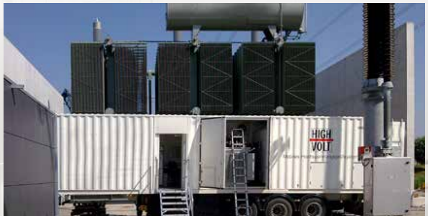
The transformer test system for on-site testing is based on the state-of-the-art frequency converter technology. The modular design and the latest digital control technology allow two or more test systems to be connected in parallel, making it possible to test even largest power transformers in the GVA range. Generally the test system can be set up on-site within an hour. There is no need for additional "lifting" or "assembly."
